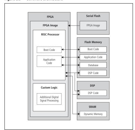
Figure 2.5 Software architecture
