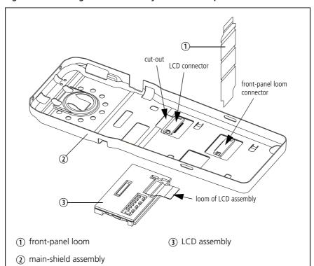
Figure 5.14 Fitting the LCD assembly and the front-panel loom
