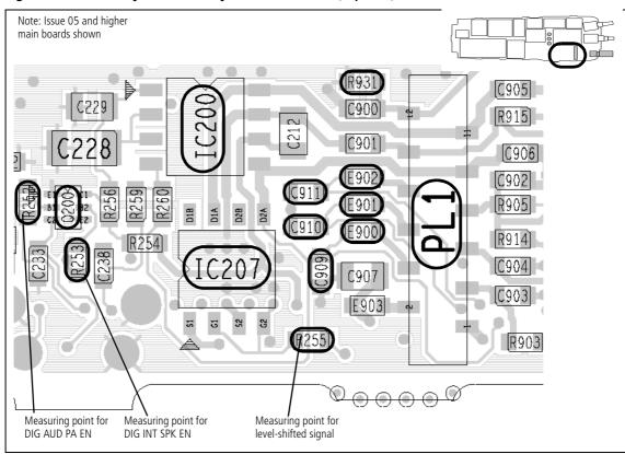
Figure 12.2 Test points for the 3V power supply and the volume potentiometer (bottom side)
