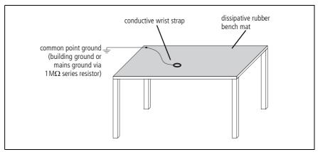
Storage and Transport of Items Always observe anti-static precautions when storing, shipping or carrying the circuit boards and their components. Use anti-static bags for circuit boards and anti-static bags or tubes for components that are to be stored or shipped. Use anti-static bags or trays for carrying circuit boards, and foil or anti-static bags, trays, or tubes for carrying components.
