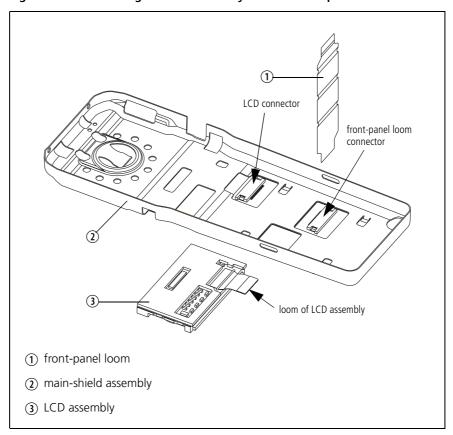
Removing the Rear Panel and the Flexible Accessory Board The circled numbers in this section refer to the items in Figure 5.7.
