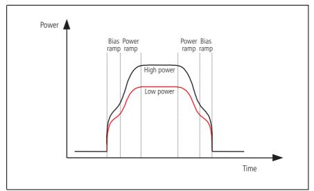
Figure 2.8 Typical ramping waveforms
