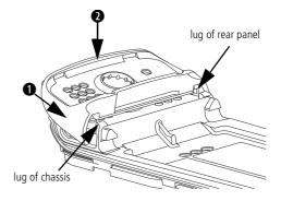
If applicable, fit the dummy cover ① and turn the lock counter-6. clockwise by a quarter turn.
