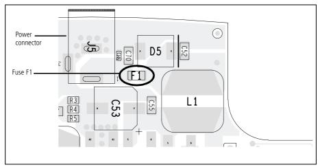
Figure 15.1 Desktop charger main board showing fuse F1 (top side)
