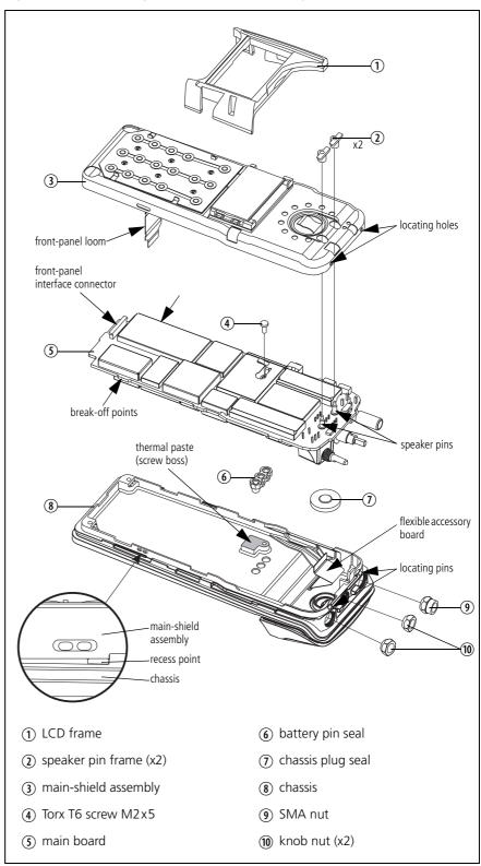
Removing the LCD Assembly and the Front-Panel Loom The circled numbers in this section refer to the items in Figure 5.6.
