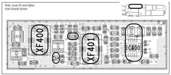
Figure 11.2 Receiver circuitry under the LO2 TOP can (top side)
