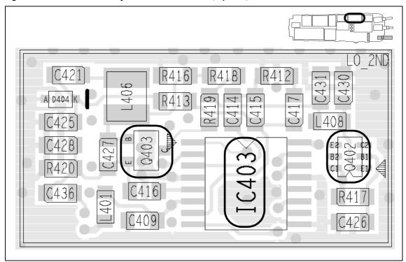
Figure 11.3 Receiver circuitry under the RX FE TOP can (top side)
