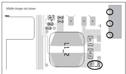
Figure 15.3 Multi-charger main board showing fuse F1 (top side)
