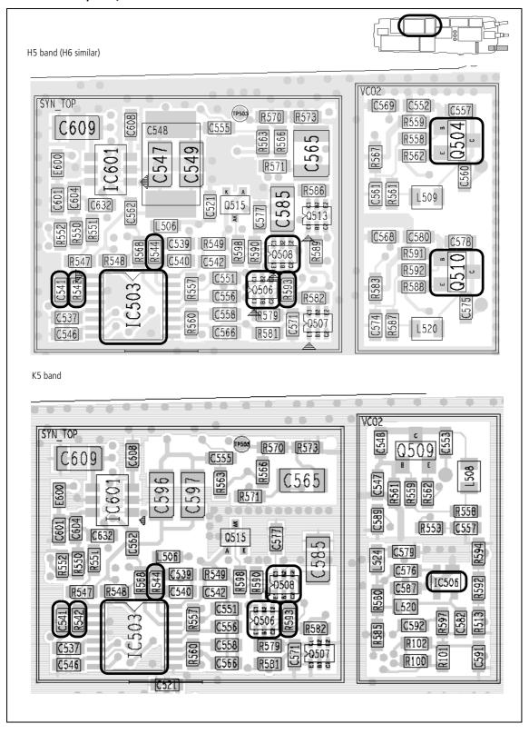
Figure 9.12 Synthesizer components under the MIXER TOP can (UHF and 800 MHz radios, top side)
